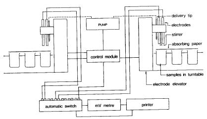
FIGURE 2 Block diagram of equipment assembly with two turntables.
